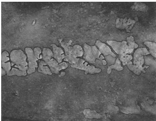
Figure 7 Disintegrated whisker after reaction with aluminium at 630° C ( \times 5000 ).
