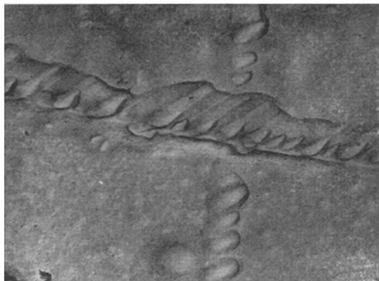
Figure 10 Replicas of whiskers after reaction with nickel at 1000° C ( \times 6500 ).
